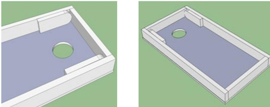
5. From the inside of the box, make a mark in the center of the 2x4 vertically inside the radius. Use the drill bit to drill a hole through the support leg and side of the box.
