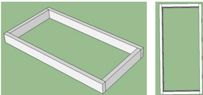
3. Lay one piece of the 24"x48" plywood on top of the 2x4 box, use the plywood to square up the 2x4 frame. Screw the plywood onto the frame with 1 5/8" screws
