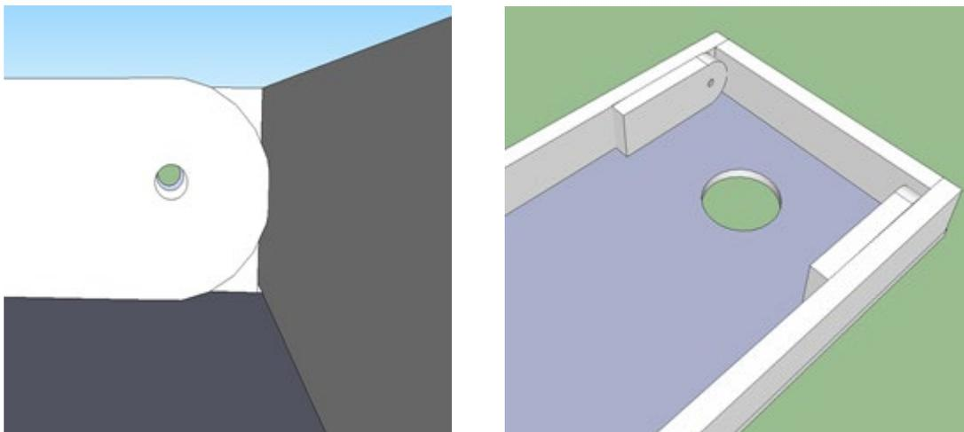
6. Install the carriage bolt through both holes and attach with a washer and a wing nut. Be sure the head of the bolt faces the outside of the box and that the washer and wing nut are on the inside.
