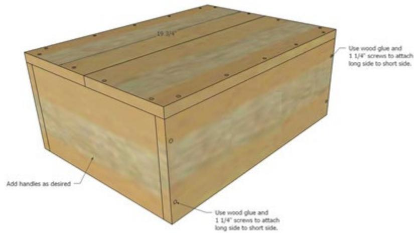
Remove any excess glue. After the glue has dried, sand the carrying crate smooth, especially the top/bottom where the jumbo Jenga will be stacked to play the game.
